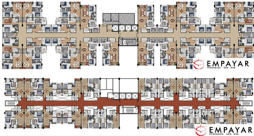
Image 6: The difference of these two floor plans can be seen with the presence of voids in bottom image which act as air wells for ventilation, while top image has covered corridors which are air-conditioned.
